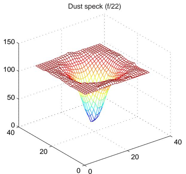
**Fig. 3.** Intensity loss due to dust speck (f/22)
