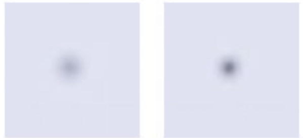
Fig. 2. Dust specks with different apertures, f/22(left), f/32(right)
