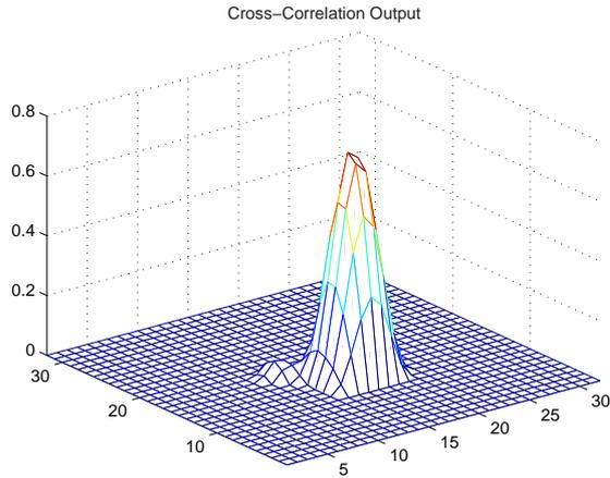
**Fig. 6.** Cross-correlation output of dust speck in fig. 4
