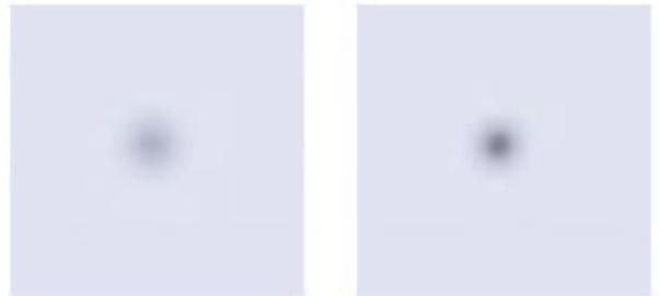
**Fig. 2.** Dust specks with different apertures, f/22(left), f/32(right)
