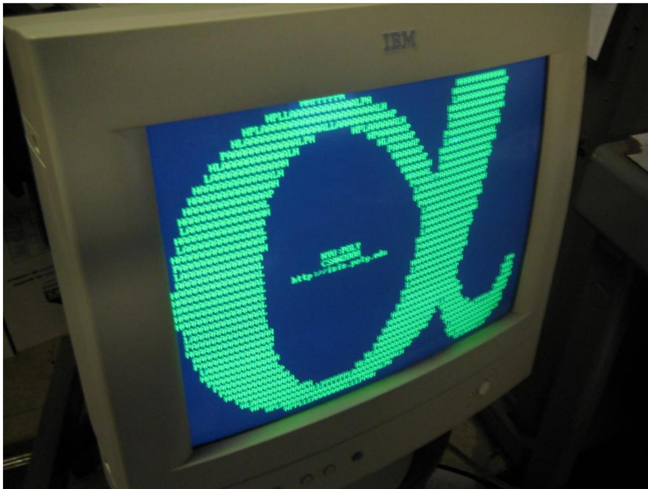
The blue carrier data is hidden by running it at frequencies close to the horizontal sync, the only visible portion is a slight bluish tint of the background color. On the monitor in test, it was very difficult to perceive the color difference.
